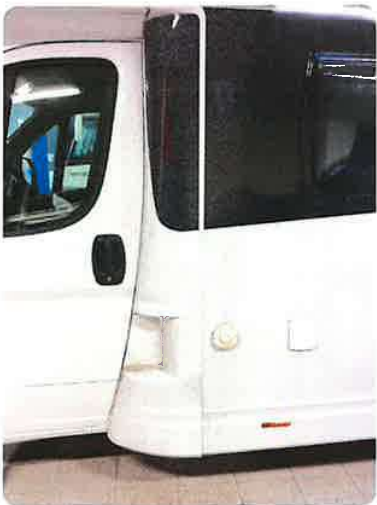
2.3 Sprekk Sprekk b-stolpedeksel v/s
